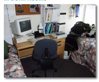
These post-fire photographs of dorm rooms show the difference a sprinkler makes. There is little visible damage in the top photo that had a sprinkler in the room; there was no sprinkler in the dorm room in the bottom picture. The dormitory burn experiment was conducted by the National Institute of Standards and Technology (NIST) and the USFA.
